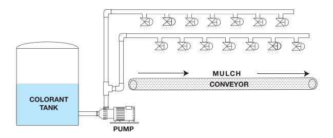
This mixer has 2 banks of 7 valves controlling the on/off function of large diameter orifice spraying nozzles. The system runs at approximately 30 psi and is supplied by a simple storage tank system and single pump.
